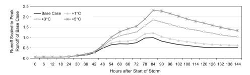
Fig. 13 Change in direct runoff due to increasing contributing area of watershed Springer
