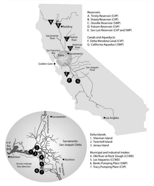
Fig. 1 State water project and Central Valley project with delta highlighted
