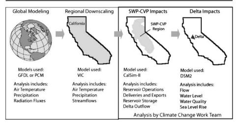
Fig. 6 Approach for analyzing potential water resources impacts of climate change
